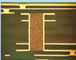
Multi-layered HDI PCB (cross-section)
