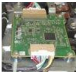
World's first inverter/converter/battery control PCB for mass-produced BEV
