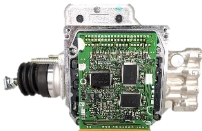
World's first PCB for regenerative braking system for HEV
