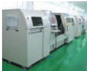
Laser hole drilling machines
