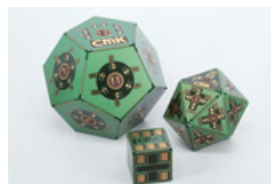
PWBs in 3D structures (high density and small dimensions)
