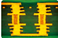
Stacked Via structure
